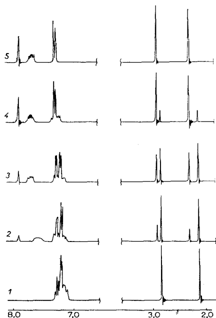
Fig. 1. PMR spectra of 1-methyl-2-acetyloindole [1] at the start of the reaction; 2) after 24 h; 3) after 3 days; 4) after 10 days] and of 1-methyl-3-acetyloindole (5) in trifluoroacetic acid.
